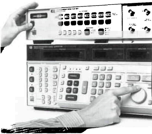
Figure 5.8. Using CAPTURE—LOOP TUNE to center the sources in the loop holding range.
